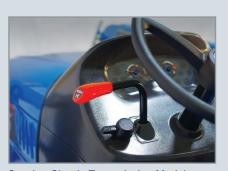
Synchro Shuttle Transmission Models Makes changing direction easier than competitive non-shuttle gear models. 12 forward / 12 reverse gear transmission provides more operating speeds than others in its class for superior control, precision and safe operations for virtually any application
