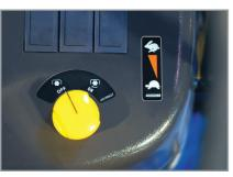
PTO On/Off switch Best easy and safety Independent PTO control with electric on/off switch. User friendly design and location for simple PTO operation.
