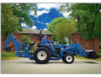
Optional quick attach backhoe Remove or attach in seconds. With 76" digging depth, 2,817 lbs of digging force and 180° swing arc, it outperforms other in its class
