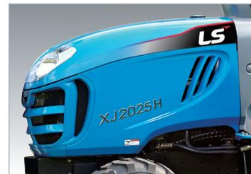
Sloping hood design improves operator view of the front end
