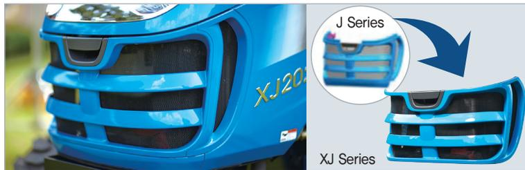
Upgraded grill design reduces foreign material from entering the engine compartment, helps prevent clogging of the radiator and engine overheating
